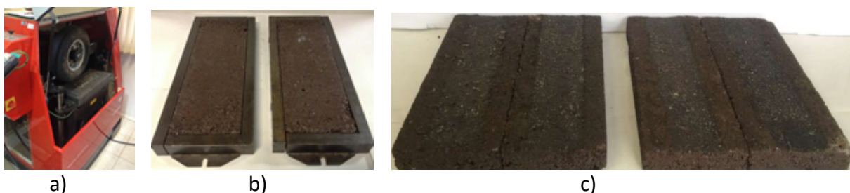
Figure 6: Permanent deformation test - a) equipment; b) samples before the test; c) samples after the test.
