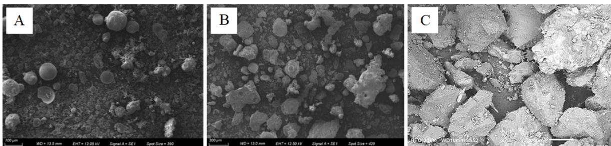
Figure 2: Scanning electron microscopy (A) Fly ash, (B) Bottom ash, and (C) Gneissic rock particles.
