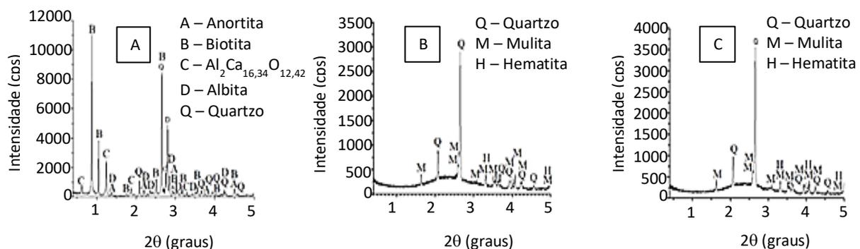
**Figure 3: XRD mineralogical analysis (A) Stone dust, (B) Fly ash, and (C) Bottom ash.**
