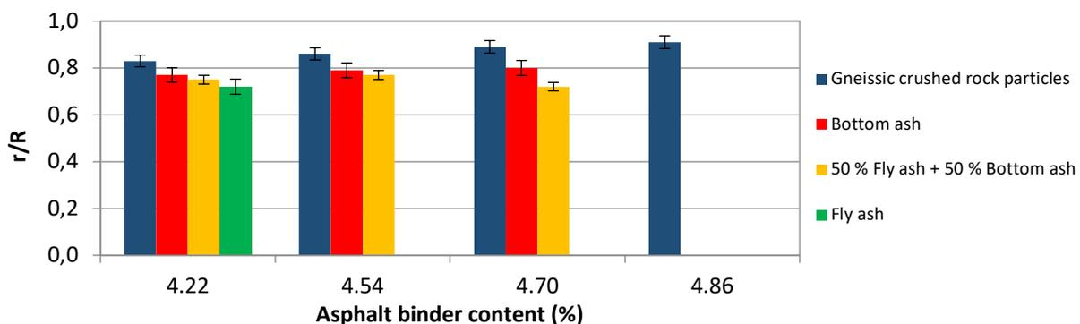
Figure 5: Results of Duriez tests.
