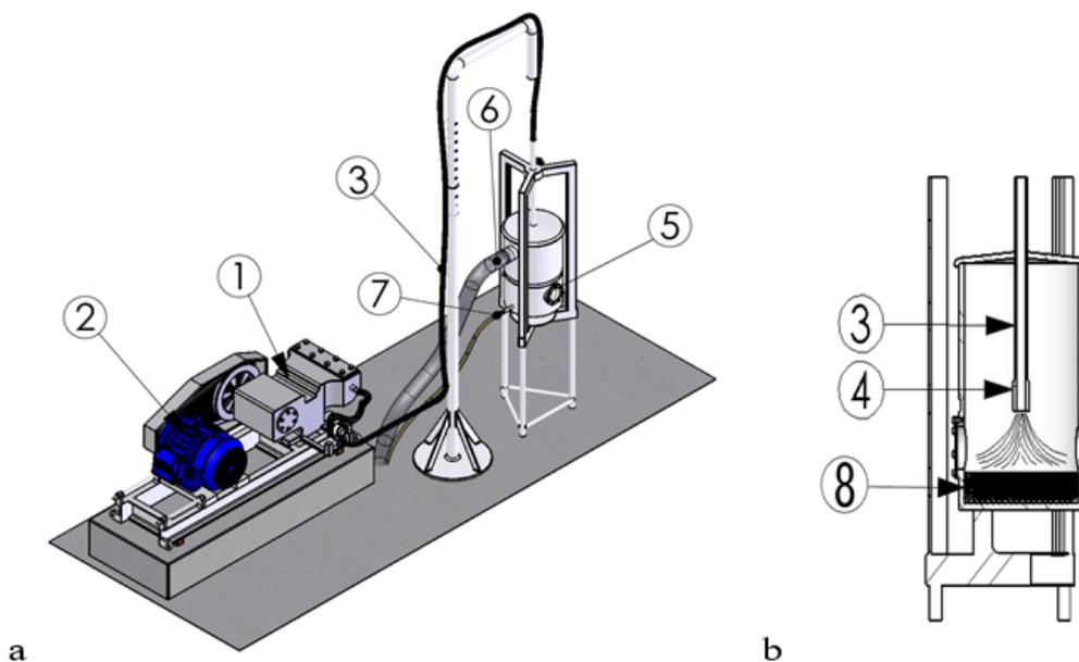
Figure 1: CJA; (a) Scheme of cavitating jet apparatus, (b) Cylindrical test tank detail (dimensions not to scale)
