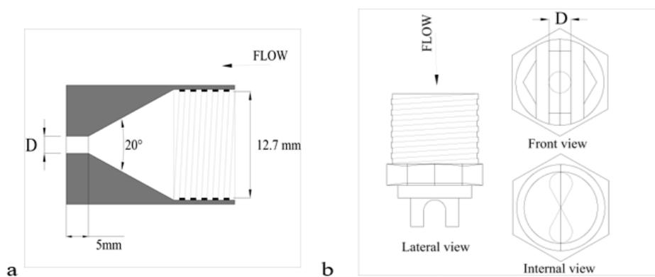
**Figure 2: Nozzles' scheme used in cavitation jet apparatus; (a)  $20^\circ$  conical nozzle, (b) MEG 2510 WASH JET SPRAY NOZZLE**
