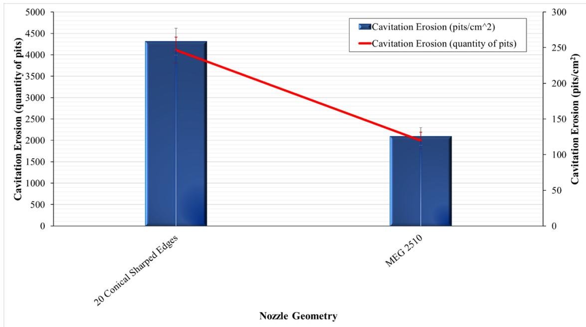
Figure 4: Effect of different nozzle geometries on Cavitation Erosion quantity at the particular moment of 1200 sec (standoff = 5 cm, orifice diameter of nozzle = 2 mm, and intensively cavitated diameter of sample = 4 cm).
