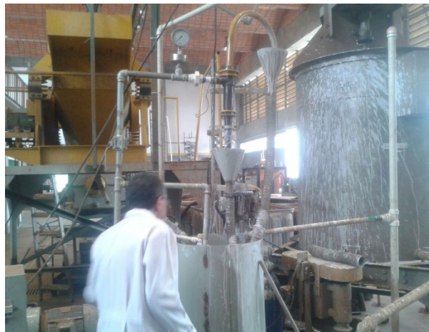
Figure 5: Hydrocyclone test for kaolin processing.
