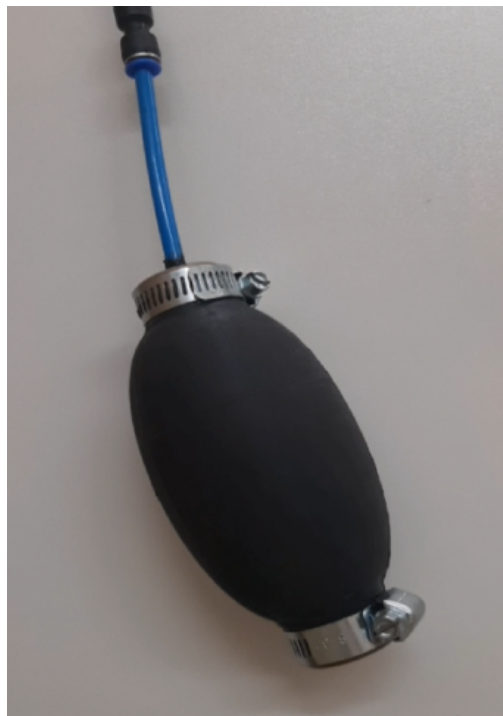
Figure 3: Inflated test probe, developed to work in confined situation at high pressure levels
