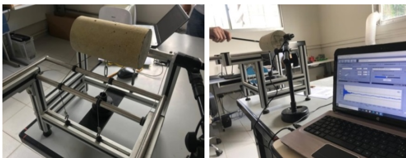
Figure 4: Dynamic modulus test.
