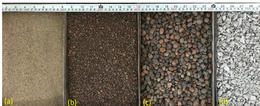
Figure 1: Comparison between the granulometries of the aggregates used: (a) natural sand; (b) AE0500; (c) AE1506; (d) gravel nº 1 (DMC 12.5 mm).
