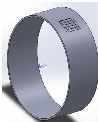
Figure 4 - Pressure vessel modeled with external corrosion.
