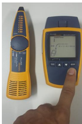
Figura 32: Sonda IntelliTone e MicroScanner
